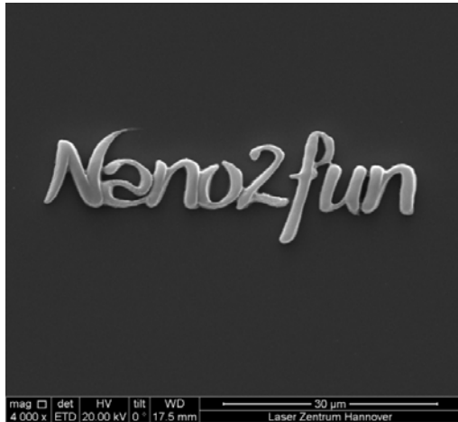
Figure 3. Scanning electron microscope image of the structure fabricated during practical training on 2PP.
