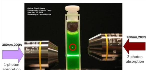
Figure (from UCF-CHEM): The one-photon (bottom of the cuvette) and two-photon absorption processes (top of the cuvette); the red circle
